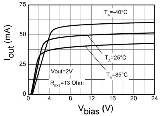
Fig. 12 Output Current vs. V<sub>bias</sub>
