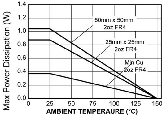
**Fig. 2 Derating Curve**
