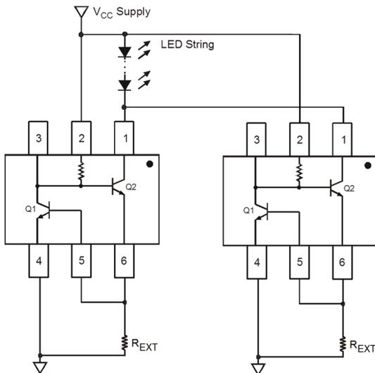
Fig. 15 Application Circuit for Increasing LED Current
