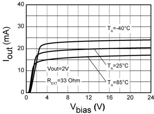
Fig. 11 Output Current vs. V<sub>bias</sub>
