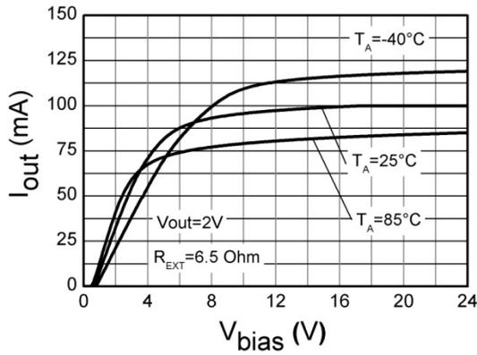
Fig. 13 Output Current vs. V<sub>bias</sub>
